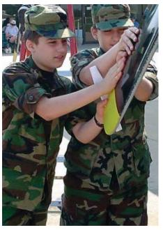
Sam and Matt carefully turn the propeller of a B-17 to clear the engine and prepare it for startup. The airplane was on its way home from an air show and stopped at Emporia to refuel.
